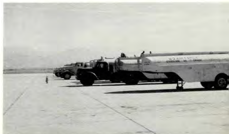
There is a 100-mesh strainer in the nozzle of the truck fill-stand hose line, above, which should be inspected according to T. O. 12-1-10. Note these trailers are parked in an open area, away from aircraft, and extinguisher is handy.
